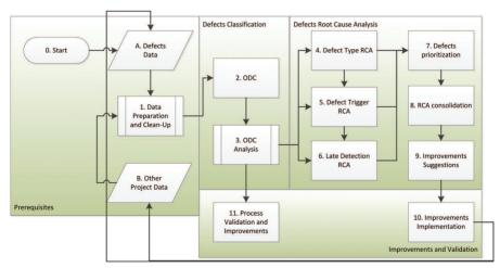
Figure 4.2 Generalized defect assessment procedure.
