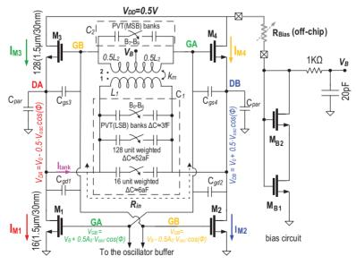
Figure 6.7 Schematic of the switching current-source oscillator.
