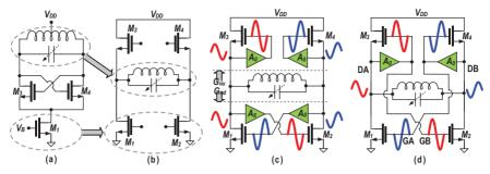
Figure 6.5 Evolution towards the switching current-source oscillator.
