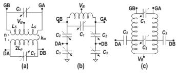
Figure 6.6 Various options of a tank providing voltage gain.
