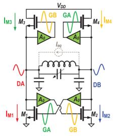
Figure 6.11 Simplified schematic of the switching current-source oscillator.
