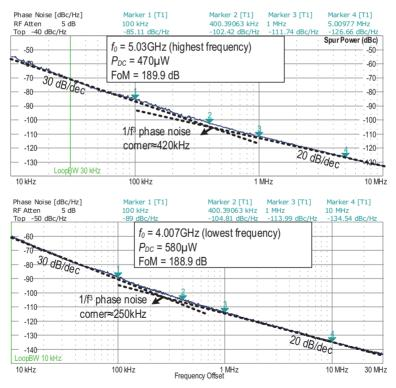
Figure 6.17 Measured phase noise of this oscillator.
