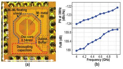
**Figure 6.16** (a) Chip micrograph; (b) measured oscillator phase noise and FoM at 3-MHz offset frequency across the tuning range.
