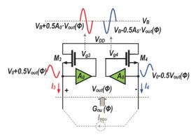
Figure 6.13 Simplified schematic of the upper pair of the oscillator.
