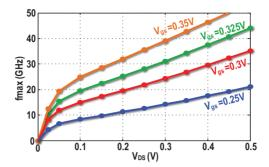
**Figure 6.9**  $f_{max}$  of low- $V_t$  28 nm transistor versus  $V_{DS}$  for different  $V_{GS}$ .
