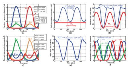
**Figure 6.14** Circuit-to-phase-noise conversion across the oscillation period in the switching current-source oscillator. Simulated (a) channel conductance of  $M_{1-4}$ ; (b) conductance due to resistive losses; (c) noise factor due to losses; (d) transconductance of  $M_{1-4}$ ; (e) effective noise factor due to transconductance gain; (f) effective noise factors due to different oscillator's components.
