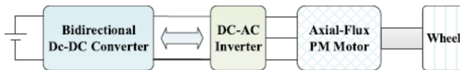
Fig.1 Use of Bi-Directional DC-DC Converter in EVs [3]
