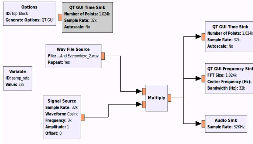
Figure 4 GRC block on GNU Radio for DVB-AM modulation technique.
