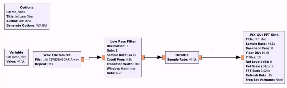
Figure 7 GRC block on GNU Radio for audio processing for gender identification.
