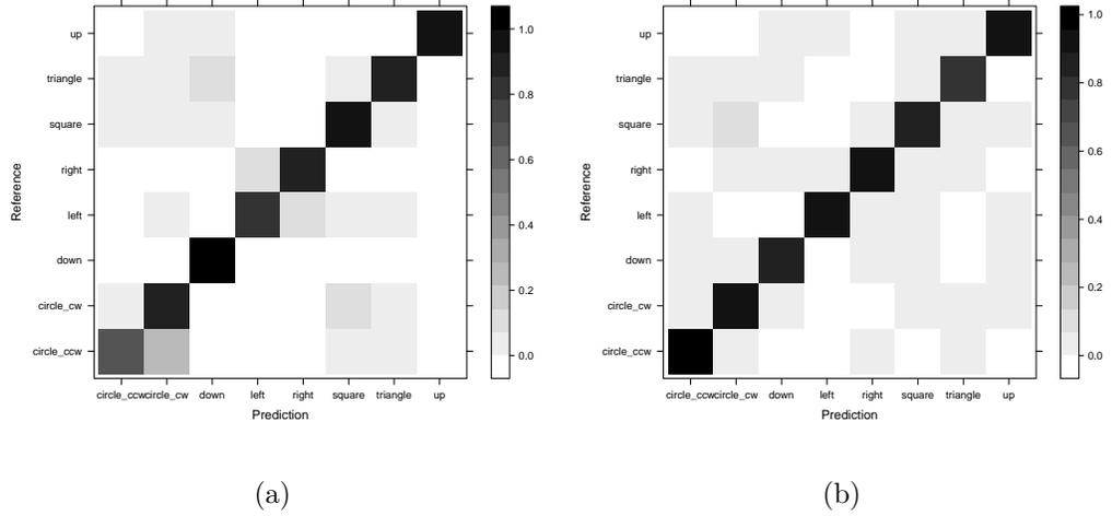
Fig. 8. The confusion matrices for the first variant of the recorded gestures with leave-subject-out cross-validation for the best classifier of (a) the Myo armband (kNN with  $k=9$ ) and (b) the LG G Watch (kNN with  $k=7$ ) with only the selected features.
