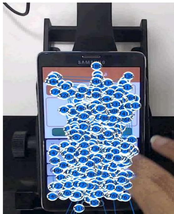
Figure 11 Picture showing the even distribution of Gaze plots while typing
