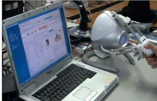
Figure A3 *Launching an application associated with the selected icon.* The system presents a reaction force through the FALCON device when the user touches the icon. He/she can launch the application by pushing the selected icon with resisting the presented force by the FALCON device. Internet Explorer is selected and launched in this example.
