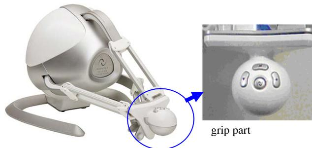
Figure 3 FALCOM force feedback device by Novint Technologies.
