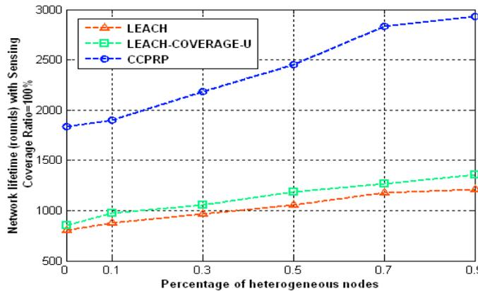
Figure 9 Comparison of the percentage of heterogeneous nodes versus the network lifetime with 100% sensing coverage ratio of the CCPRP protocol with those of other protocols.
