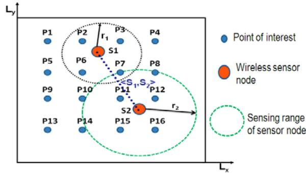
Figure 2 Example for the coverage model of sensor nodes.
