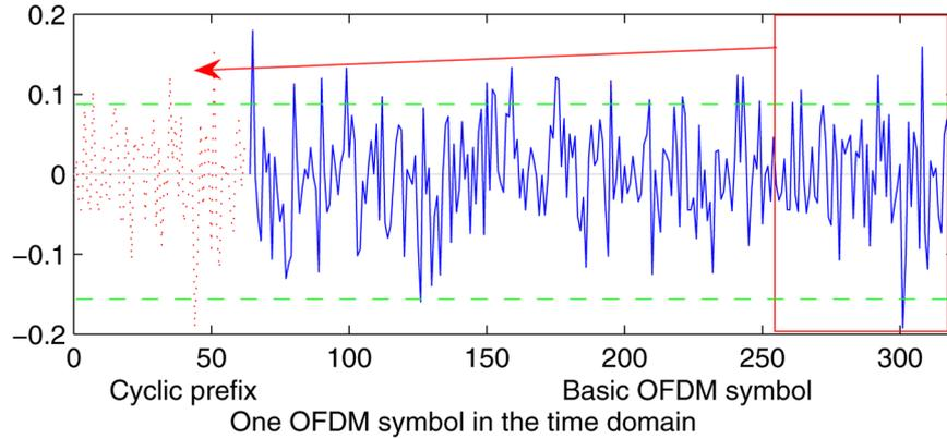
Figure 3 Time domain representation of an OFDM symbol, dotted line – cyclic prefix, solid line – basic OFDM symbol.
