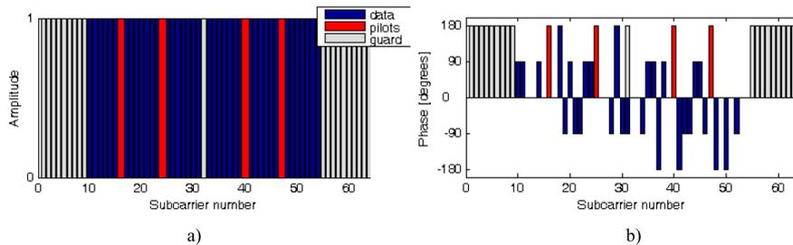
Figure 2 Frequency domain representation of one OFDM symbol: (a) amplitude of subcarriers, (b) phase of subcarriers.
