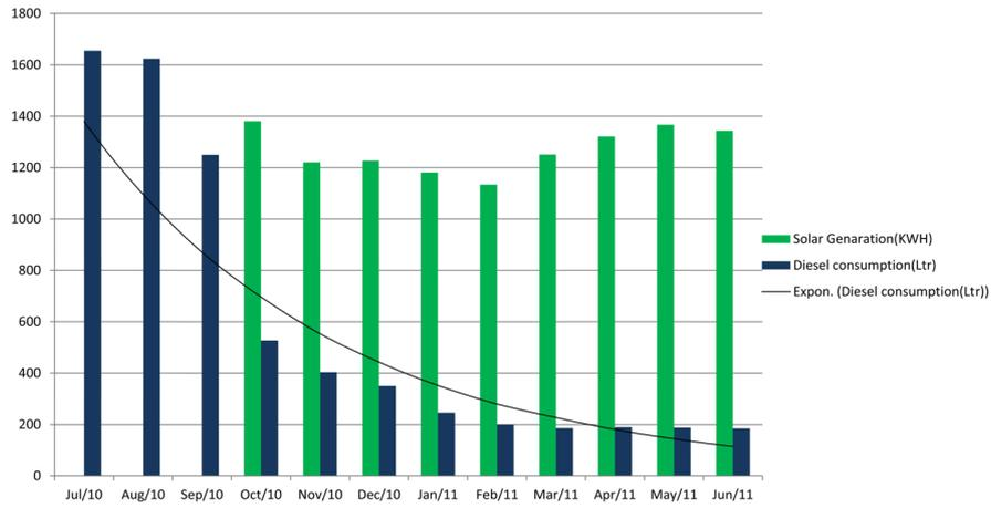
Figure 5 Trend of monthly reduction of diesel consumption and increase in solar generation.
