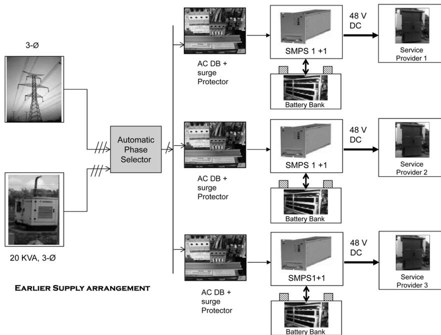
Figure 1 Schematic diagram of the existing power distribution arrangement.
