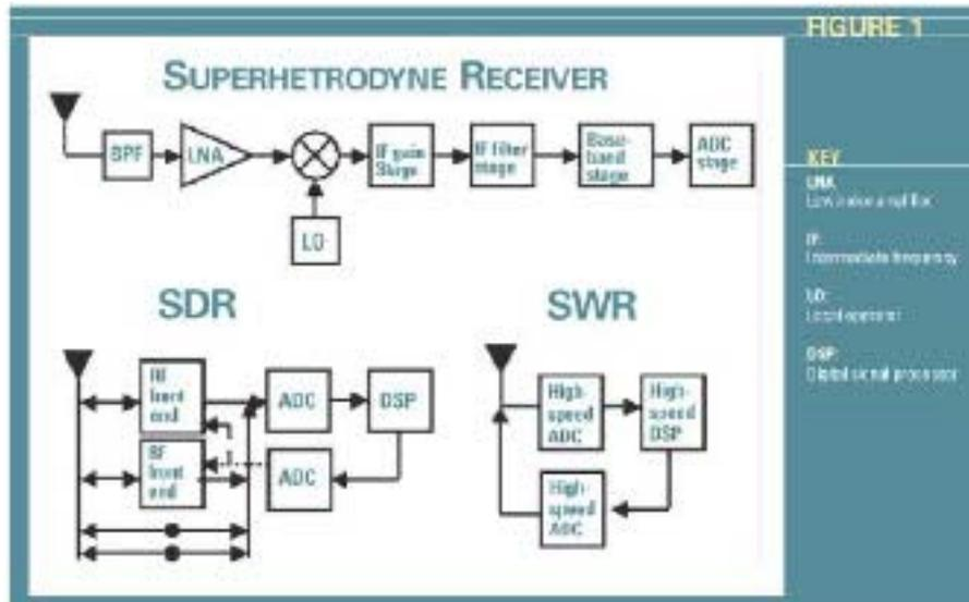
Figure 1 Software defined radio (SDR) versus software radio (SWR).
