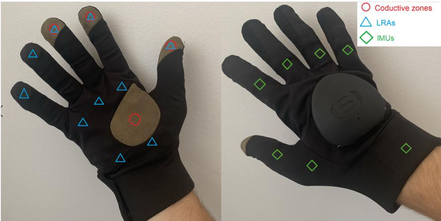
Figure 15.2 Sensors and actuators of Sensorial XR [16].
