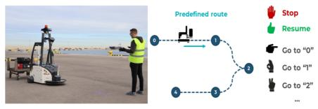
Figure 15.6 On-site cockpit implementation (left) and route control schema (right).
