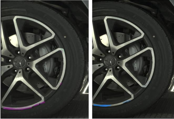
**Figure 11.5** Rim damage detection example (target – left; result – right).
