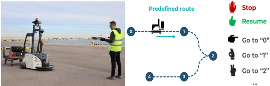
**Figure 15.6** On-site cockpit implementation (left) and route control schema (right).
