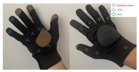
Figure 15.2 Sensors and actuators of Sensorial XR [16].
