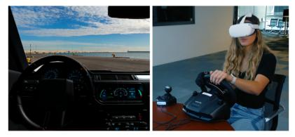
**Figure 15.5** Remote cockpit implementation from first-person view (left) and third-person view (right).
