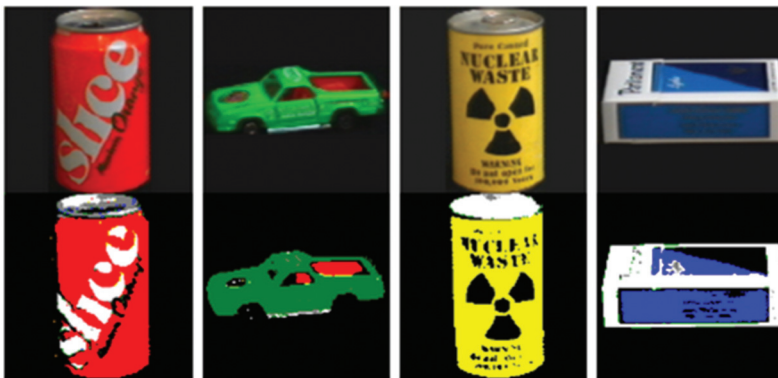
Figure 4.7 Examples of obtained visual colors’ interpretations (lower images) and corresponding original images (upper images) for several testing objects from COIL database.
