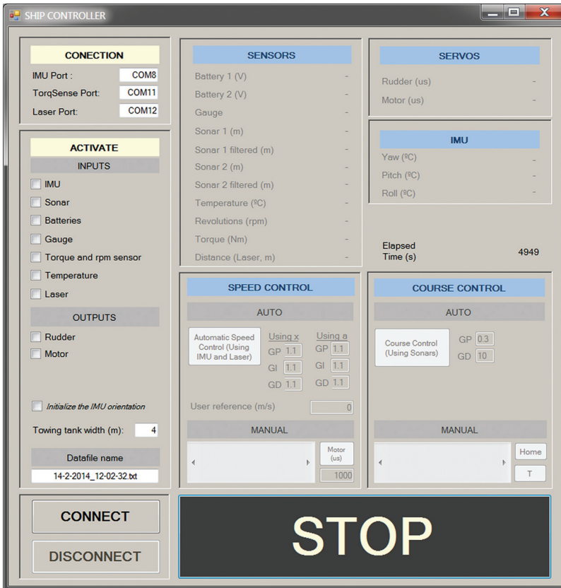
Figure 3.3 Graphical user interface to monitor/control the model from an external workstation.
