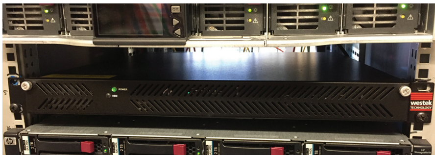
Figure 9.5 IP-based digital exchange for ship-to-shore radio anno 2016.
