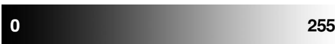
Fig7. Image gradient showing pixel values going from very dark: black (0) to lighter: white (255).
