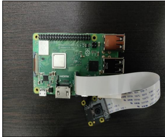
Fig.6. Raspberry Pi 3 B+ and NOIR IR camera.
