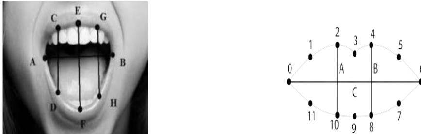
Fig 4.5.1 & Fig 4.5.2. Landmark indices for mouth region The formula to estimate the Mouth Aspect Ratio (MAR) is given below:
