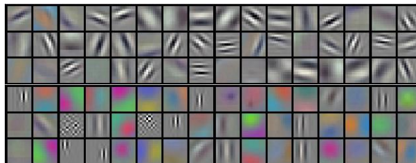
Fig6. The above image shows the Example of the image feature detectors that a CNN might "learn" during its training.
