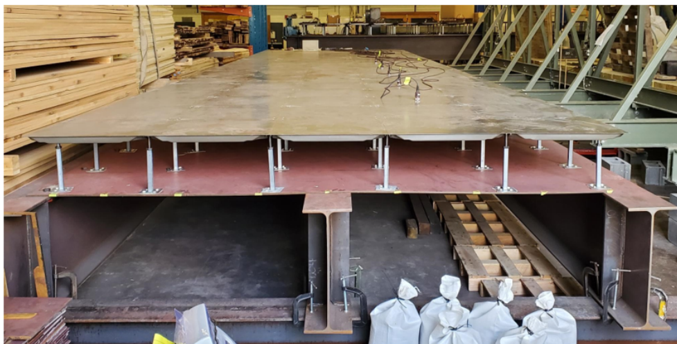
Fig. 1 The light specimen (SM68_RAF) with W24 \times 68 beams, a 3/8 in. thick plate, and raised access floor (RAF).
