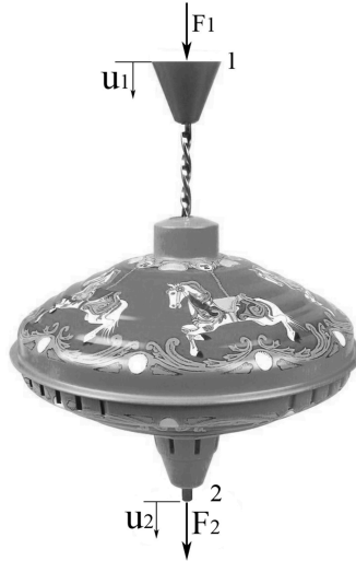
Fig. 1 A physical realization of the inerter in which the force output is proportional only to the relative acceleration between nodes 1 and 2.
