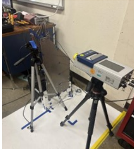
Fig. 7 Comparison setup with LDV and neuromorphic camera.
