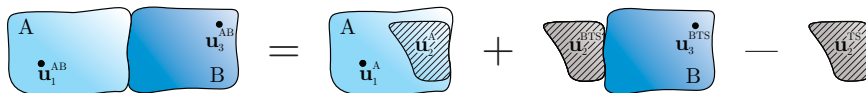
Fig. 2 Coupling application with a TS substructure. Common interface for all substructures is presented as hatched.
