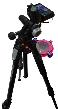
Fig. 8 Set-up for image capture for DIC. A camera on a tripod was used to photograph the polymer with fine speckled pattern.
