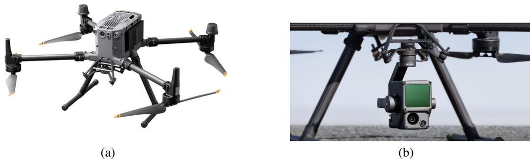
Fig. 1 DJI Matrice 350 RTK (a), and L1 Zenmuse LiDAR sensor (b).
