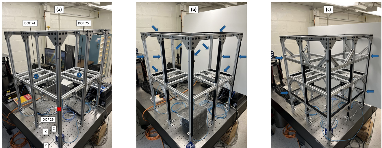
Fig. 1 The three test stand configurations: (a) undamped, (b) damped, (c) stiffened
