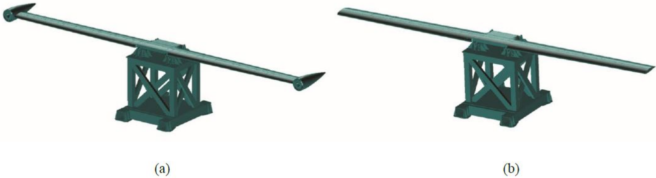
Fig. 9 Finite element model for the X-57 Mod III wing on the wing loads test fixture for configuration A (Fig.9a); and configuration B (Fig.9b).
