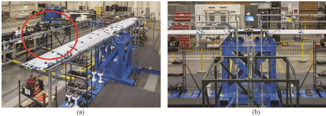
Fig. 10 Aileron actuation mechanism in front of the X-57 Mod III wing (Fig. 10a); and close-up view with the cables attached (Fig. 10b)
