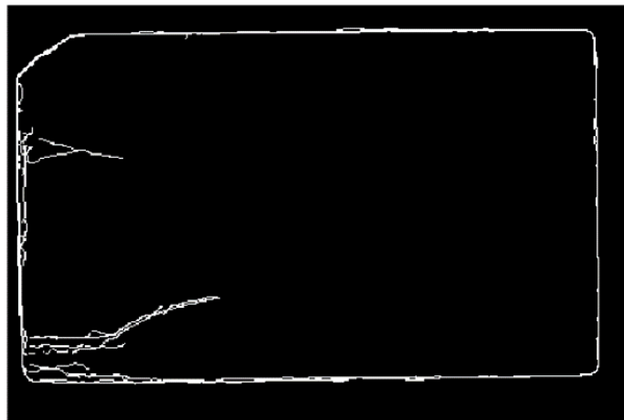
Fig. 10 Composite binary image of a wafer with cracks displaying both wafer edges and cracks present within the bounding geometry. This image is produced by applying Canny edge detection to each resonance mode scan independently and combining the resultant images.
