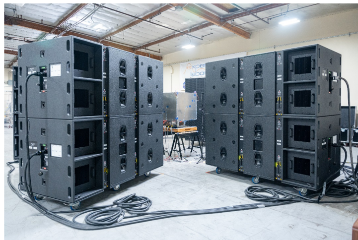
Fig. 1 Demonstration article inside 6 \times 2 configuration of ARS Neutron acoustic sources.
