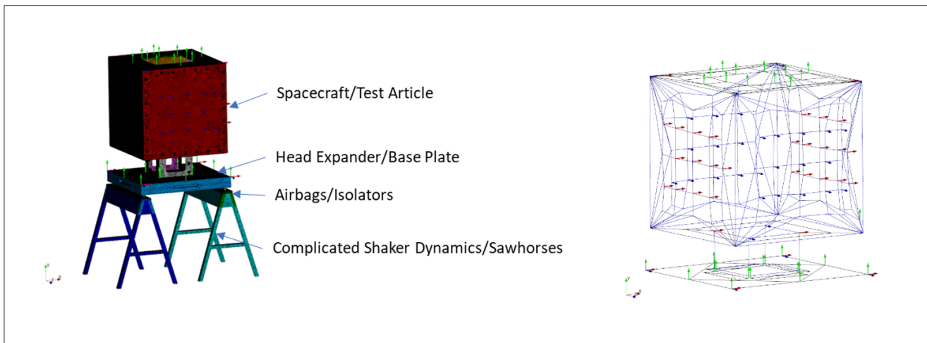
Fig. 2 FEM (left) and test display model (right) showing accelerometer locations.
