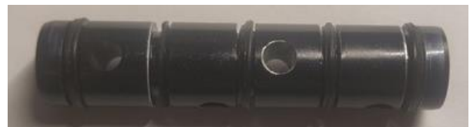
Figure 15: Spool after 733,000 cycles with visible damage to seals and control edge
