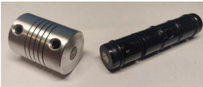
Figure 13: Breakage of the control spool at the contact with the flexible coupling at 733000 switching cycles
