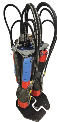
Figure 18: Humanoid legs with 2x3 rotary valves on top of the structure
