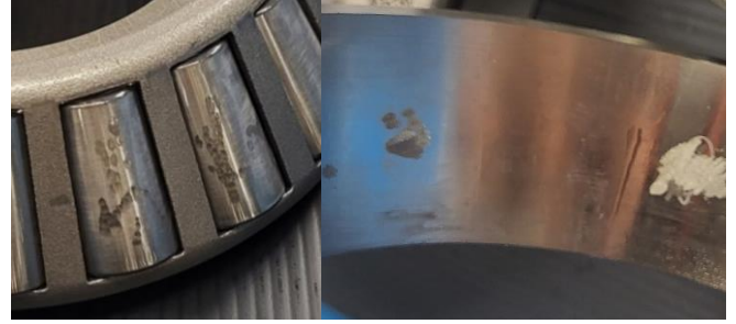
Figure 2: Manipulated roller elements (left) and outer ring (right) with abrasively generated spalls
