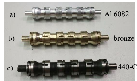
Figure 2. Prepared control valve spools: a) aluminium alloy Al 6082, b) bronze and c) hardened stainless steel AISI 440-C respectively.
