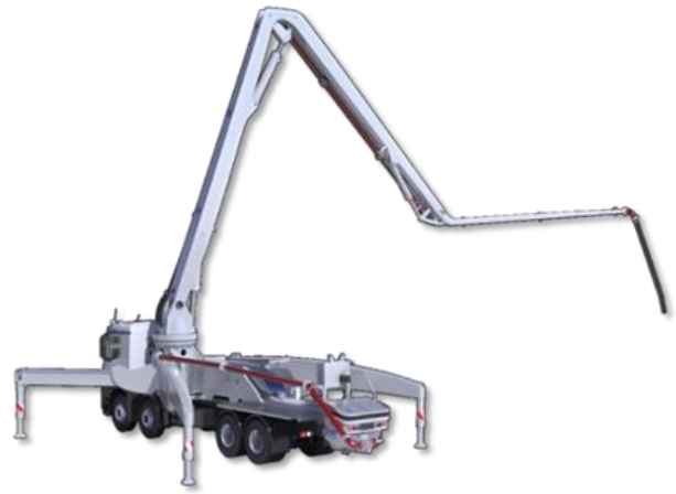
Figure 1: Concrete pumping equipment fitted with a large hydraulic manipulator.
