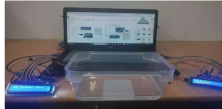
Fig 3: IR communication across the water medium
