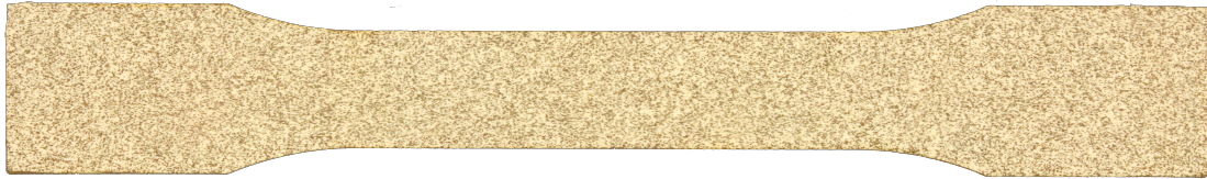
Fig. 4 Specimen with Goodman generated speckle pattern sublimated onto its surface
