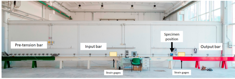
Fig. 2 Split Hopkinson Pressure Bar installed at Marche Polytechnic University
