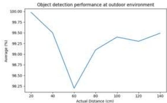
Fig. 4. Accuracy Analysis on Outdoor Object Detection
