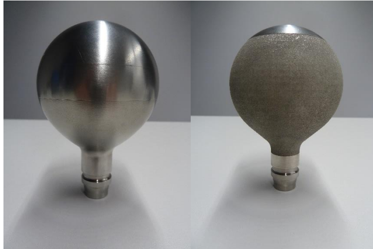
Figure 8: Helmholtz Resonator - conventional and additive manufacturing
