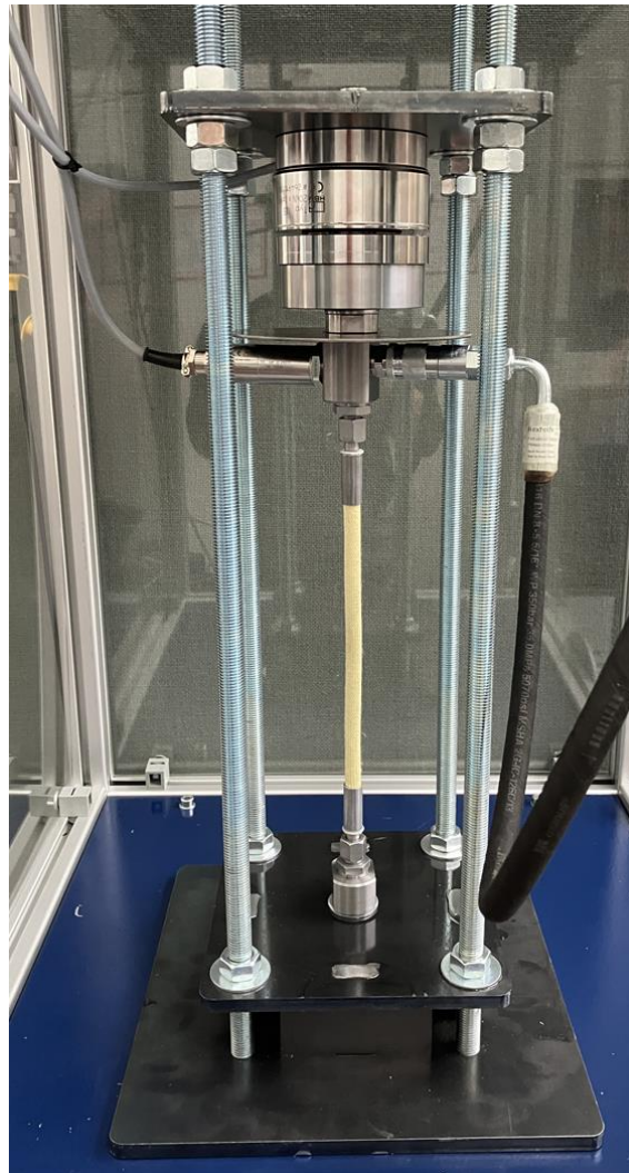
Figure 7: Measuring device to determine the maximum blocked force F_t of the clamped muscle
