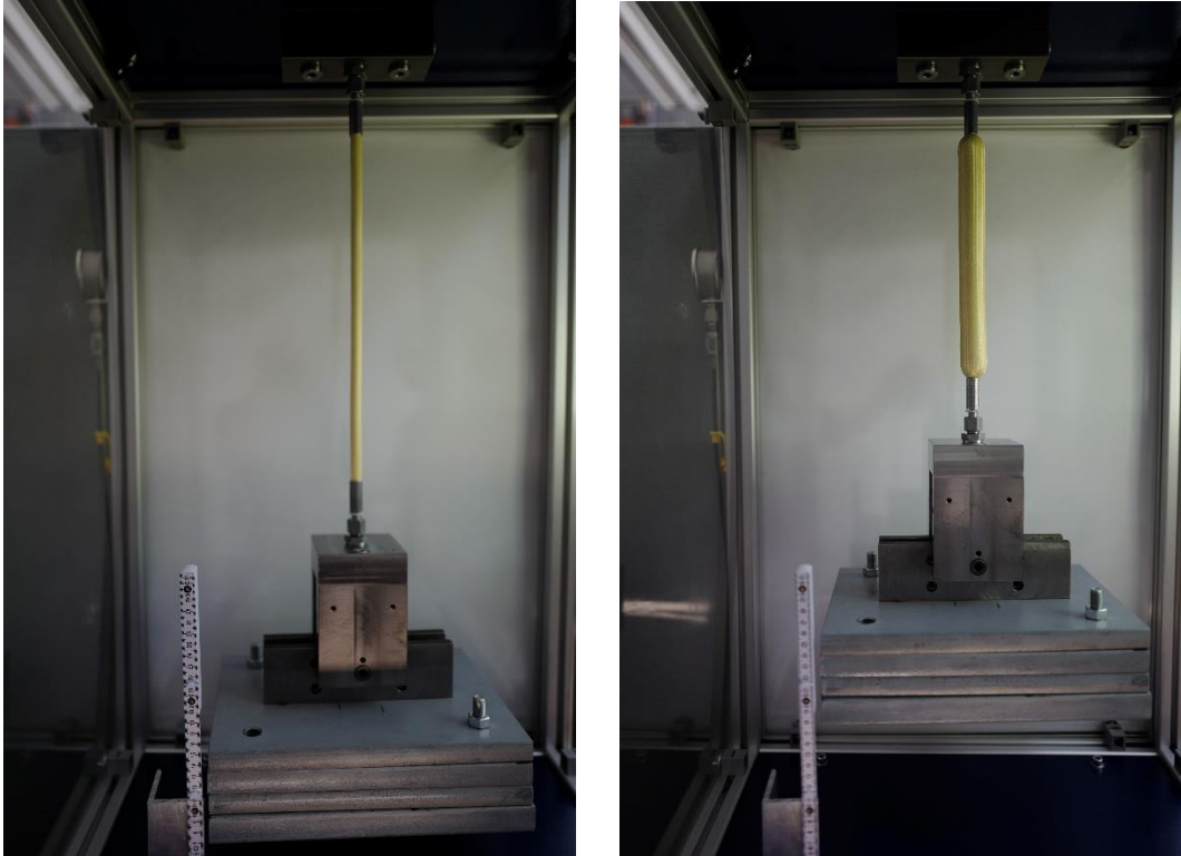
Figure 4: Hydraulic artificial muscle non-pressurized (left) and pressurized (right)
