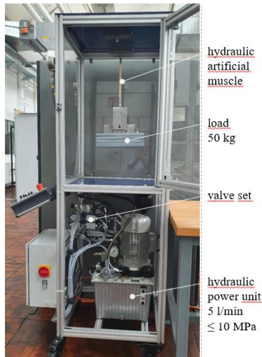
Figure 3: Hydraulic test setup for the investigation of the muscle contraction
