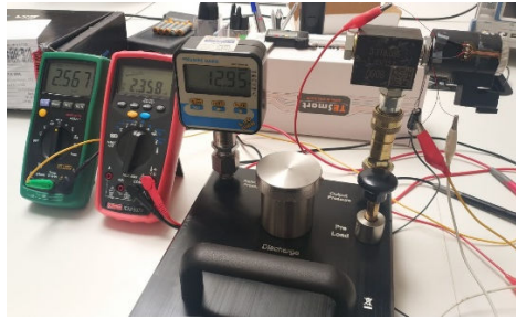
Figure 11. Static Pressure Test Bench
