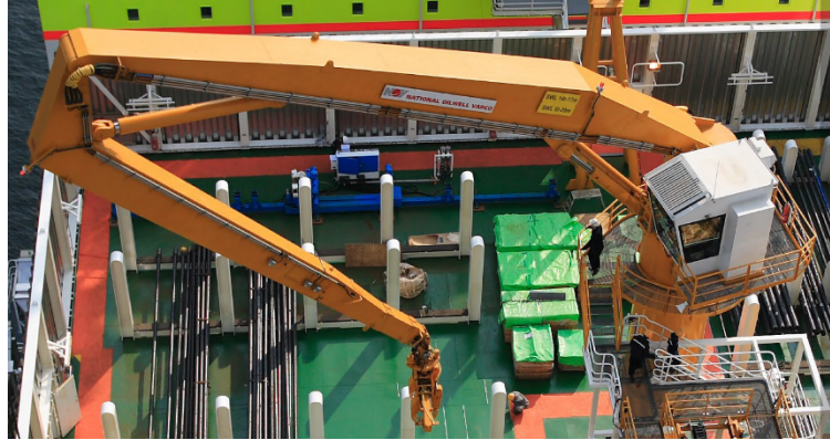
Figure 3. A PHC from National Oilwell Varco. ©
