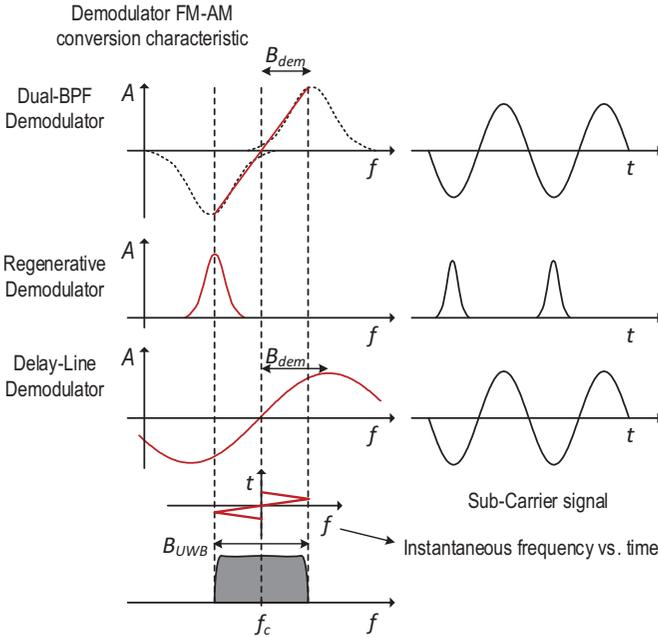
**Figure 3.10** Frequency-to-amplitude conversion characteristic of reported FM demodulators.
