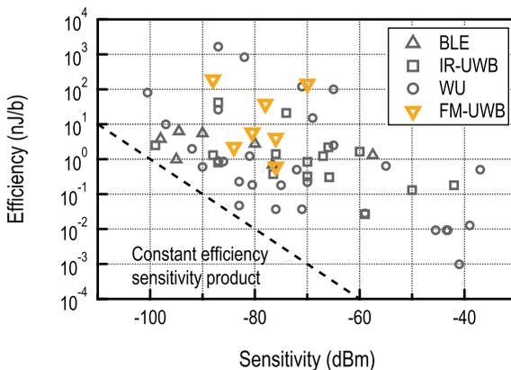
**Figure 3.12** Comparison of FM-UWB receivers and other low power receivers from Chapter 2, efficiency against sensitivity.
