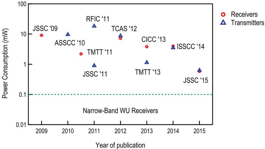
**Figure 3.13** FM-UWB transmitters and receivers, evolution of power consumption. Type of demodulator used in each receiver is indicated on the graph.
