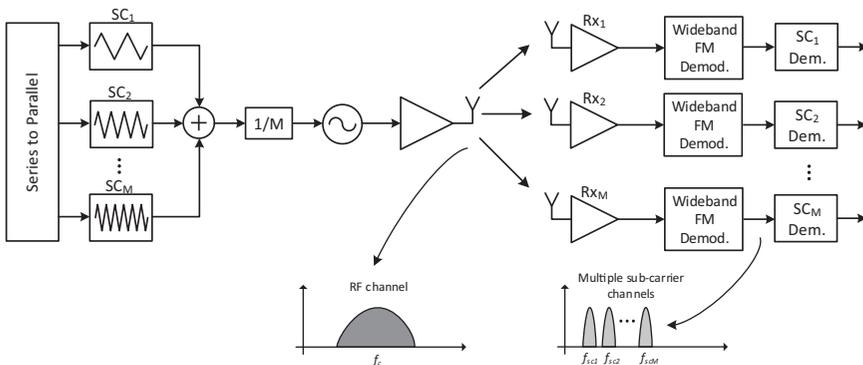
Figure 3.7 FM-UWB multi-channel broadcast.
