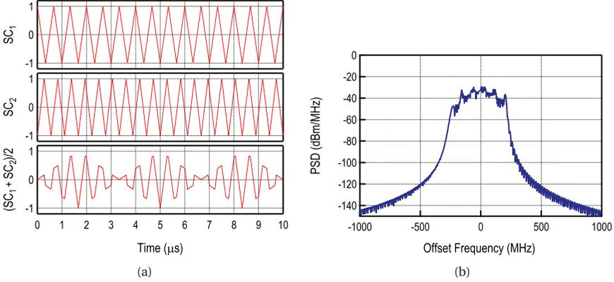
**Figure 3.8** Example of transmission on two channels, time domain sub-carrier signal (a) and transmitted signal spectrum (b).
