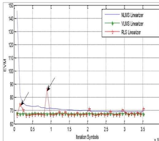
Figure 3-2 RMS-EVM analysis (V-LMS vs N-LMS & RLS)
