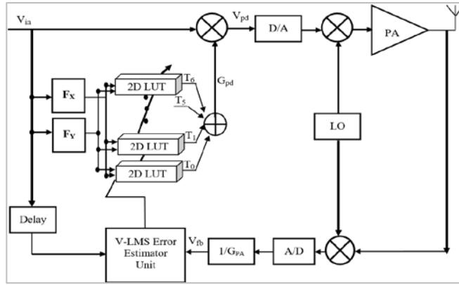
Figure 3-1 proposed Pre-Error Inclusion V-LMS Linearizer
