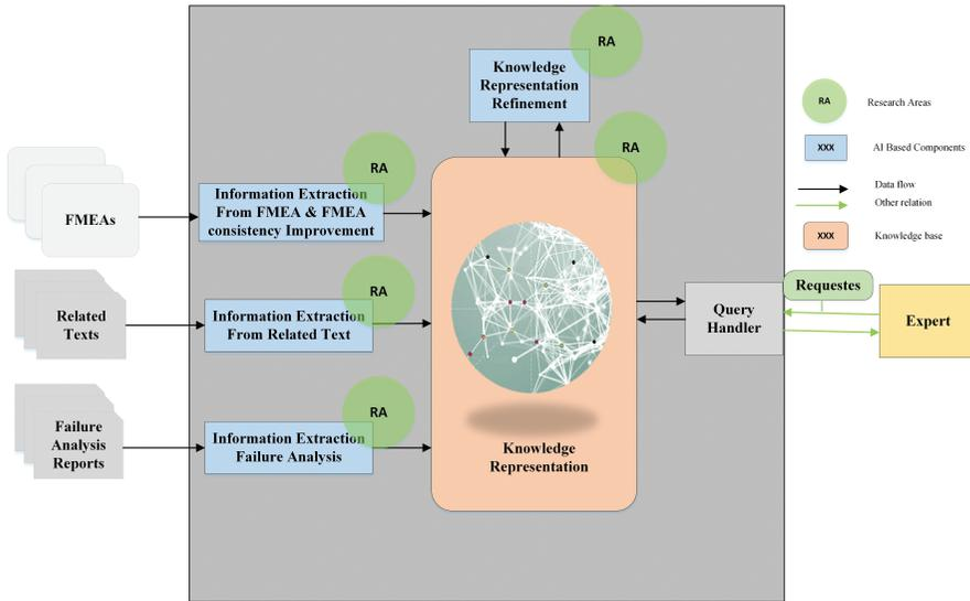
**Figure 2.1.1** AI-based knowledge management concept system for risk assessment and root cause analysis in semiconductor industry.
