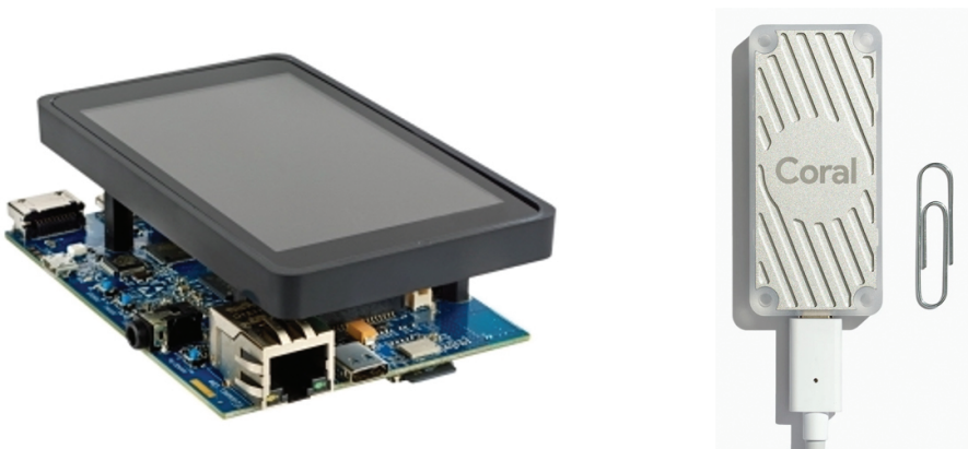
Figure 4.3.3 STM board and TPU accelerator used in this work.
