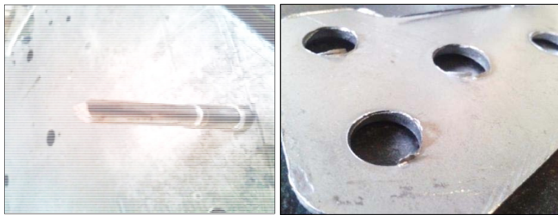
Figure 1.1 Failure of Punches as well as burr on edges of component
