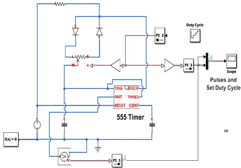
Fig 4: 555 Timer circuit diagram to generate PWM pulses
