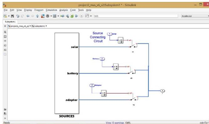
Fig 8: Connection of sources to main power circuit
