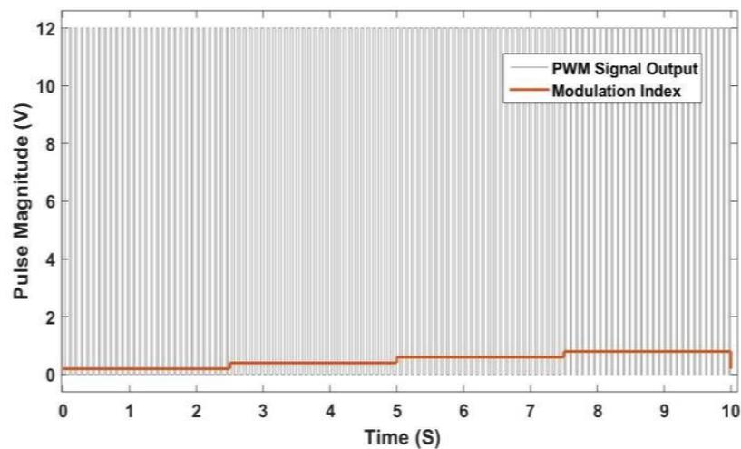
Fig 5: 555 Timer PWM pulses for different Modulation Index.
