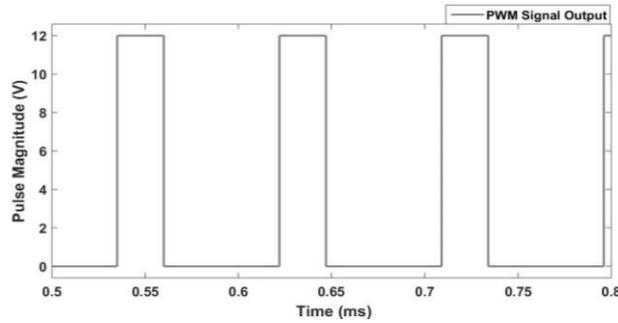
Fig 6: 555 Timer PWM pulses for 25% Modulation index.
