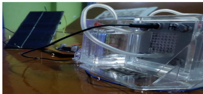
Figure 3.1. Hardware setup of Hydrogen and Oxygen production from solar PV panel using Electrolyzer 1. Solar PV panel 2. Buck Converter 3. Electrolyzer
