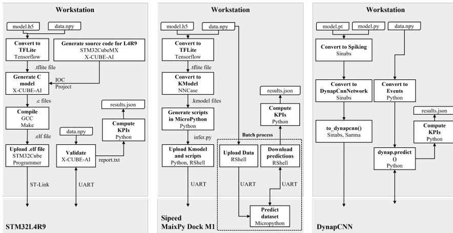
**Figure 10.2** Deployment pipelines for all platforms. From left to right: STM32L4R9, Kendryte K210 and DynapCNN. For DynapCNN, the pipeline is contained in a single Python script, while the other rely on external languages and tools.
