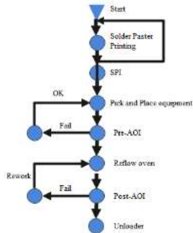
Figure 2. Process flow in considered SMT line
