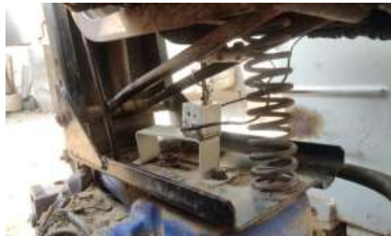
Figure 2. Location of accelerometer on the base of tractor seat.
