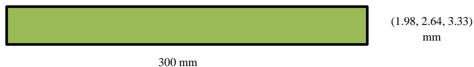
Figure 1. Geometry of Aluminium Plate
