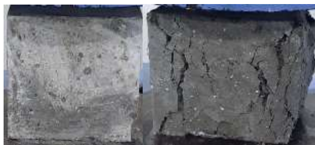
Figure 2. General crack bridging and failure mechanism
