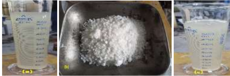
Figure 3. Raw materials (a) sodium hydroxide solution, (b) sodium hydroxide flakes, (c) sodium silicate solution
